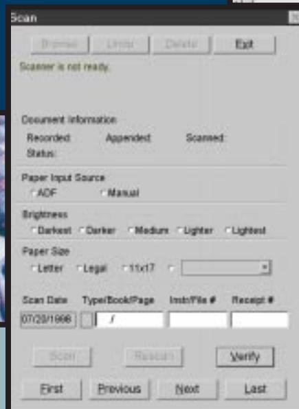
*The module allows the user to rescan pages and append pages to the record if necessary. The operator has extensive control over the scanner settings, to ensure quality.*
